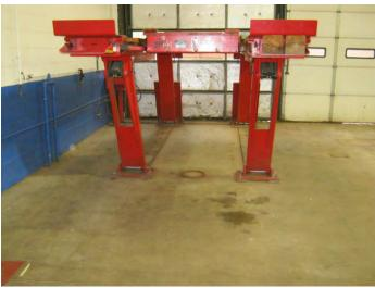
Piston (center, under aboveground lift) with associated hydraulic controls against wall (left), automotive garage.
